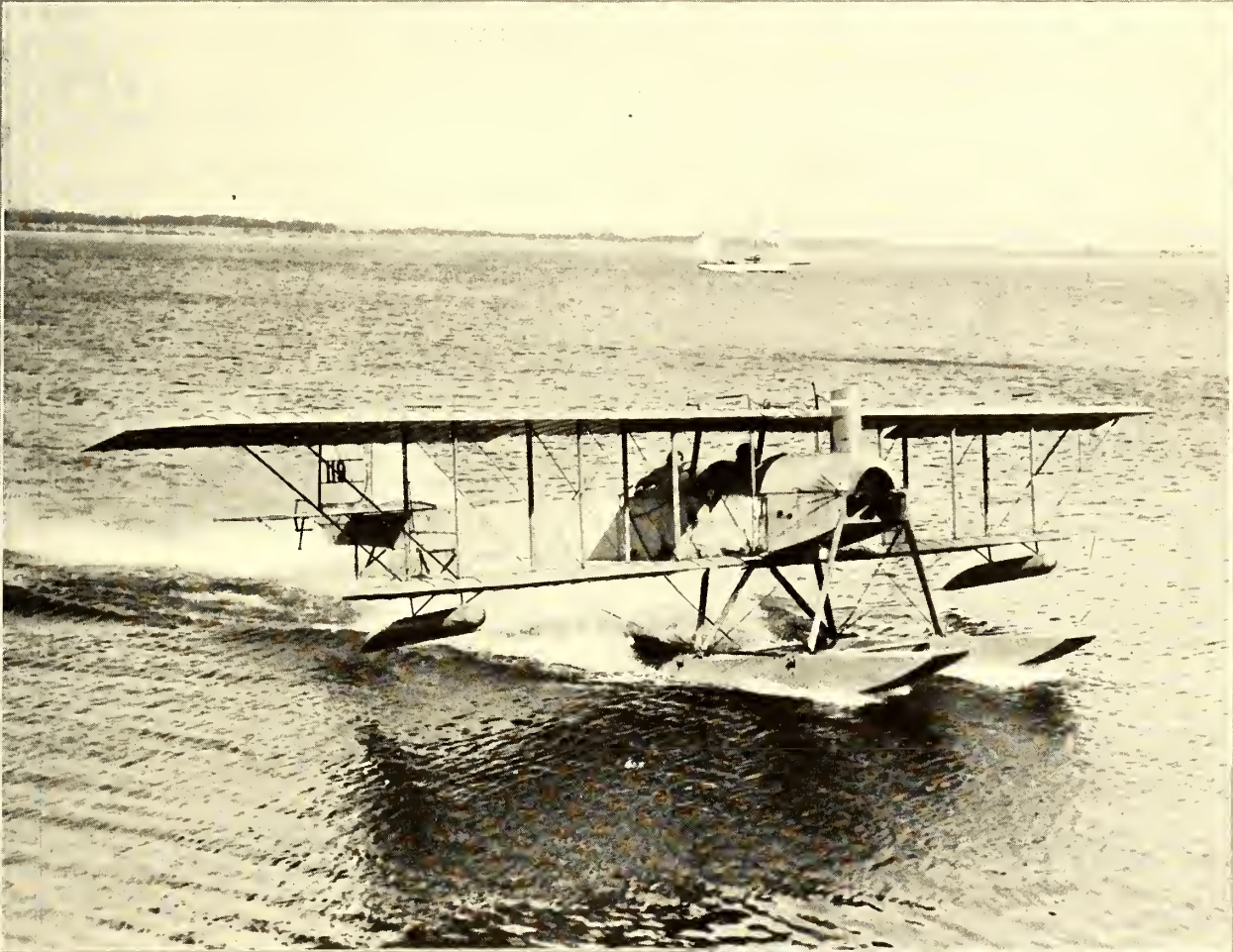
One of the Short "folders" (160-h.p. Gnome engine) taxiing home to Calshot after alighting in Southampton Water from a trip round the Fleet on Saturday. Note the funnel for the exhaust gasses.
